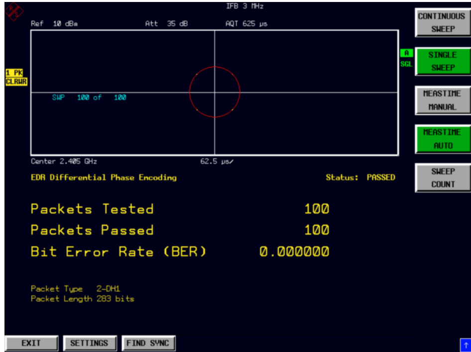
Fig. 3-13 Differential Phase Encoding (EDR) measurement
